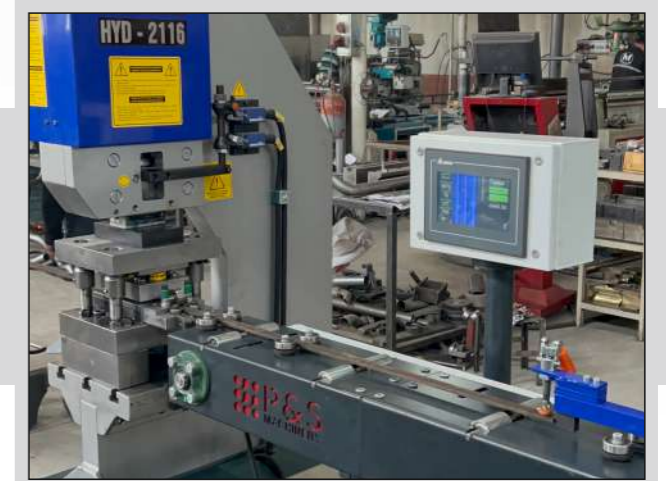
12 Metreye Kadar Otomatik Servo Besleme Sistemi Automatic Servo Feeding System Up To 12 Meters
