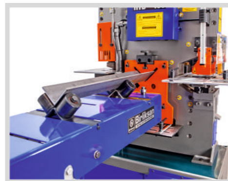
Köşebent Ve Npu Besleme İçin Makaralar Feeding Rollers For Angle Iron and NPU
